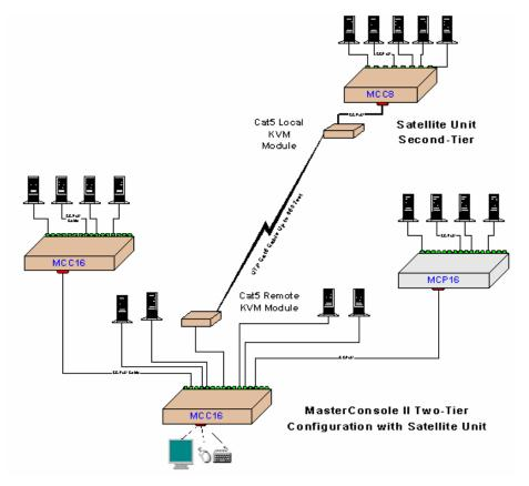
Figure 34 Two-Tier Configuration with Satellite Unit
